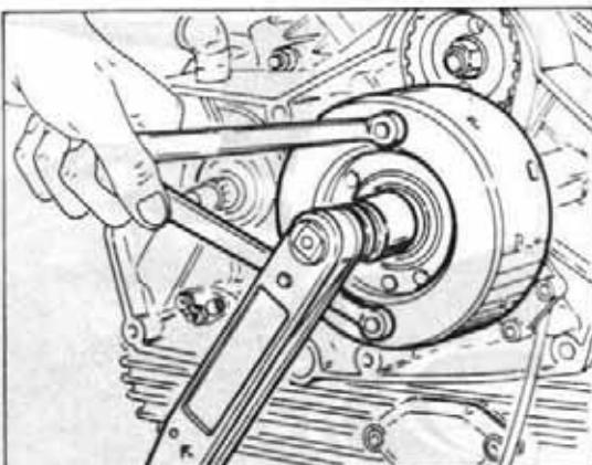
Proceed with the reassembly of the rotor, making sure that the key is correctly fitted on the crankshaft, and that the two conical surfaces (of the shaft and the rotor) have been thoroughly cleaned of oil and grease, using trichloroethylene and a clean cloth, before proceeding with the fitting of the rotor.
