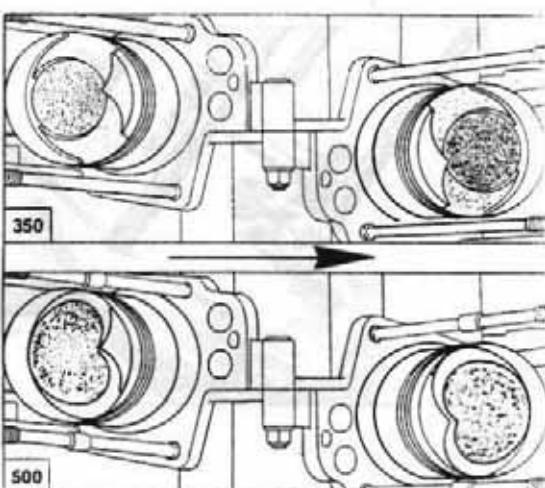
**● Pistons must be installed the correct way round. Refer to figure.**
